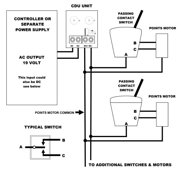
The drawings above show very simple arrangements using the CDU and two points motors. There could of course be many, many more than this in a layout.
