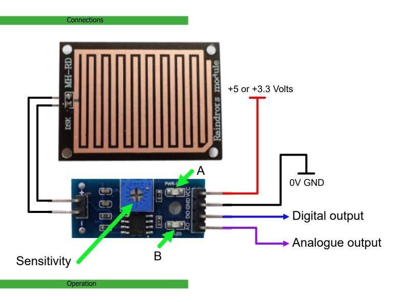
This module can be used to detect snowflakes, raindrops or just used for moisture detection.
