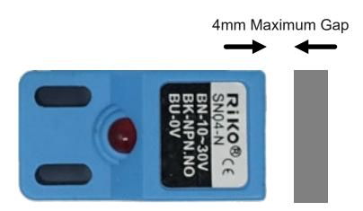
When metal passes the sensor head (within about 4mm) the indicator LED turns on and the output changes from 0 volts to the supply voltage. This could operate a relay, sound an alarm alarm or connected to another device.
