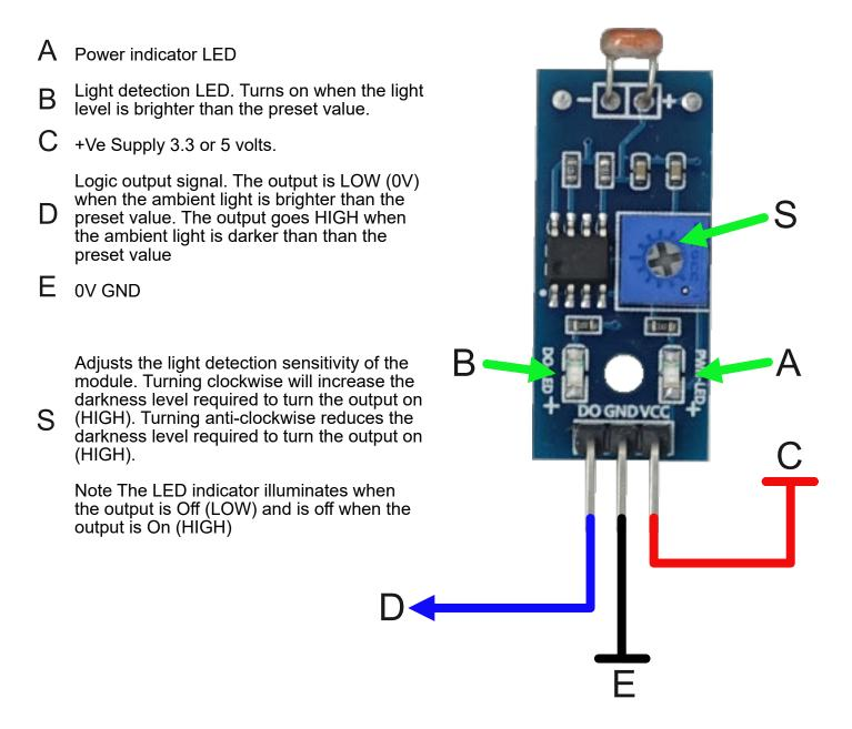
This module will detect the ambient light level. When the light is greater than the preset value the output will be LOW (0V). If the ambient light is darker than the preset value the the output goes High (either 3.3 volts or 5 volts depending on supply voltage).
