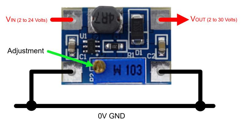
The input and output connections will need to be soldered. The bottom or the top of the board may be soldered.
