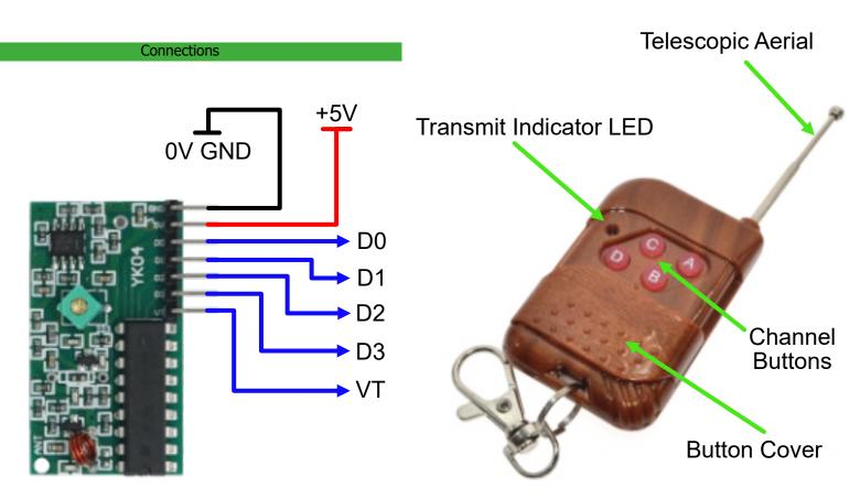
Connect GND and +5V as shown. The power supply must be a regulated DC 5 Volt power supply.
