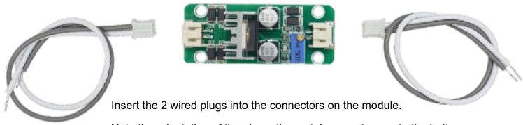
Note the orientation of the plugs, the metal connectors go to the bottom
