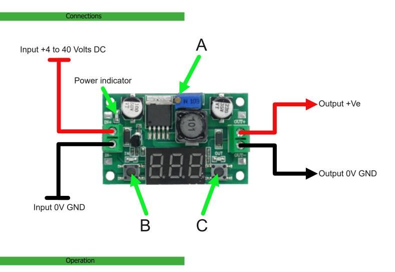
This DC to DC converter outputs a DC voltage from 1.2 Volts to 37 Volts. The input voltage must be at least 1.2 volts higher than the maximum required output voltage. I.e. if the input voltage is 12 volts then the maximum output voltage would be approximately 10.8 volts.
