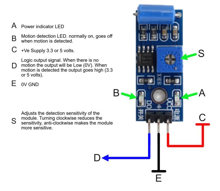
This module will detect both motion and vibration. When motion or vibration is detected the output which is normally low (0V) goes high (either 3.3 volts or 5 volts depending on supply voltage).
