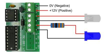
Shown are the power and 2 LED output connections.
